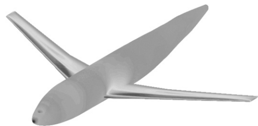
Fig. 12. Pressure contours over the DLR-F6 wing-body configuration at M_\infty = 0.75 , \alpha = 0.52^\circ , and Re = 3 \times 10^6 .
