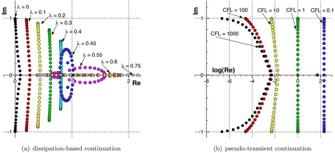
Figure 2. Discrete spectrum for various values of  $\lambda$  and CFL for a uniform grid with  $h = 0.03125$ . The  $x$ -axis in Figure (b) is the natural logarithm of the real part of the spectrum. The black-filled circles in both figures can be regarded as the spectrum of the system matrix for the unmodified problem (9).
