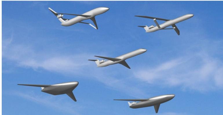
**Figure 2:** Unconventional aircraft configurations that could be critical for achieving improved fuel efficiency and reduced emissions. A conventional aircraft (centre) is surrounded by concepts for more efficient designs - clockwise from top left: box-wing configuration, strut-braced-wing configuration, lifting-fuselage configuration, and hybrid-wing-body configuration. Credits: Thomas Reist and David Zingg - University of Toronto Institute for Aerospace Studies.
