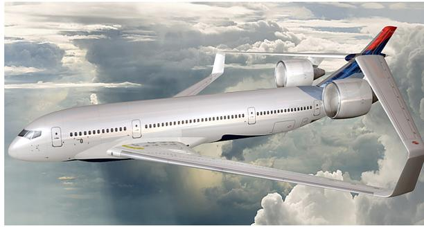
**Figure 6:** Lockheed Martin's box-wing concept for the N+2 study (source from [223]. Credits: NASA/Lockheed Martin).
