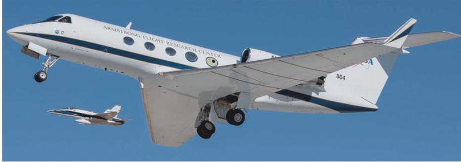
**Figure 10:** The FlexSys morphing wing geometry on a Gulfstream III flight test aircraft with no external flap-track or distinct control surfaces under the wing, source: [40]
