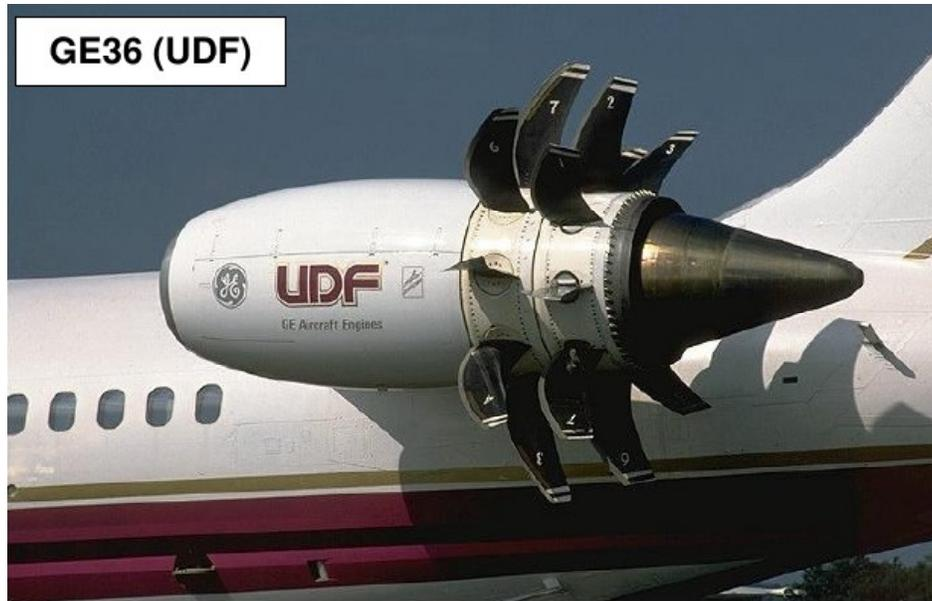
**Figure 11:** The open rotor concept (experimental GE36 engine), source: [3]
