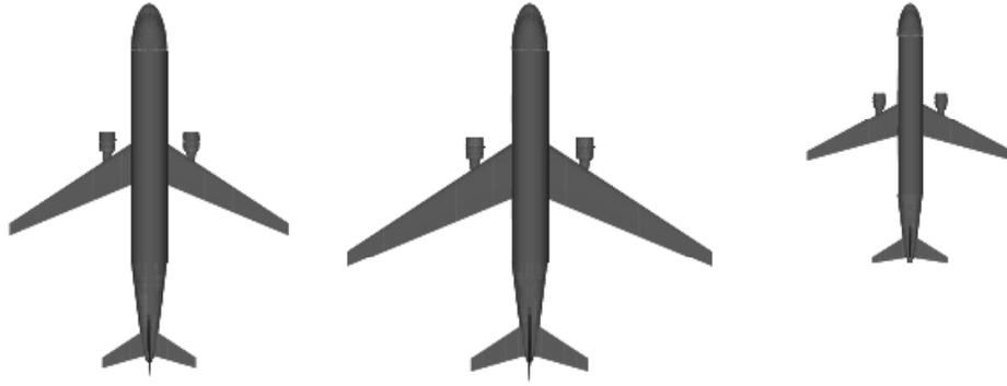
**Figure 8:** Planform view of LASR (left), A330 (center) and A320 (right), source: [63]
