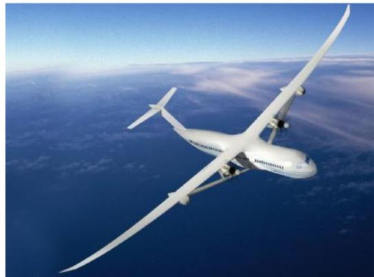
(d) Strut-braced wing design, source: [21]
