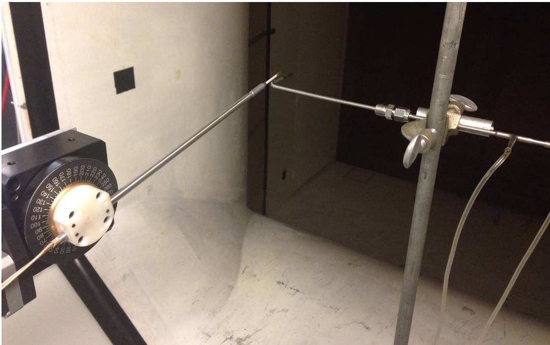
Figure B.1: Photo of the cross-wire probe during calibration.
