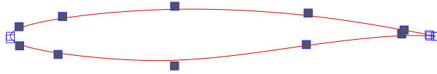
Figure 1. B-spline control points; the shaded control points are used as design variables.
