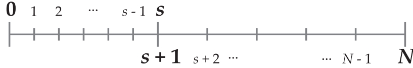
Figure 3.1: Example domain consisting of two subdomains with an interface at x_s = x_{s+1} .
