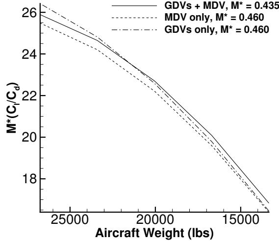
Figure 5. A comparison of UAV range performance optimized with and without Mach number as a design variable. GDV's: geometric design variables, MDV: Mach number design variable,  $M^*$ : optimal Mach number
