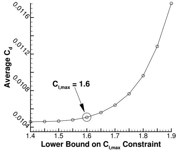
Figure 8. Trade-off between performance at cruise conditions and  $C_{l,\max}$  constraint at low-speed conditions for Design Problem 1
