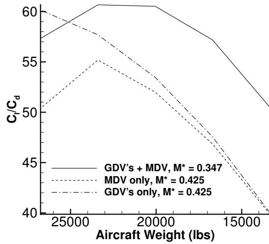
Figure 6. A comparison of UAV endurance performance optimized with and without Mach number as a design variable. GDV's: geometric design variables, MDV: Mach number design variable,  $M^*$ : optimal Mach number
