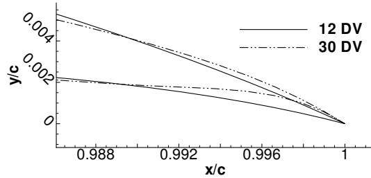
**Figure 12.** Comparison of optimized airfoil trailing edges with 12 and 30 design variables
