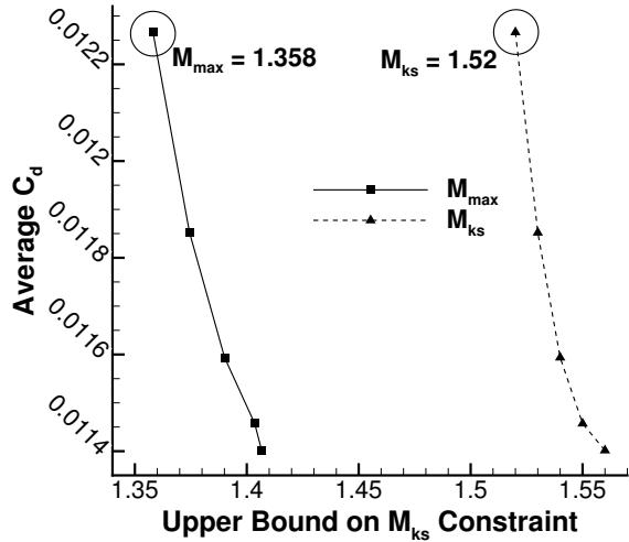
Figure 7. Trade-off between performance at cruise conditions and  $M_{ks}$  constraint at dive conditions for Design Problem 2
