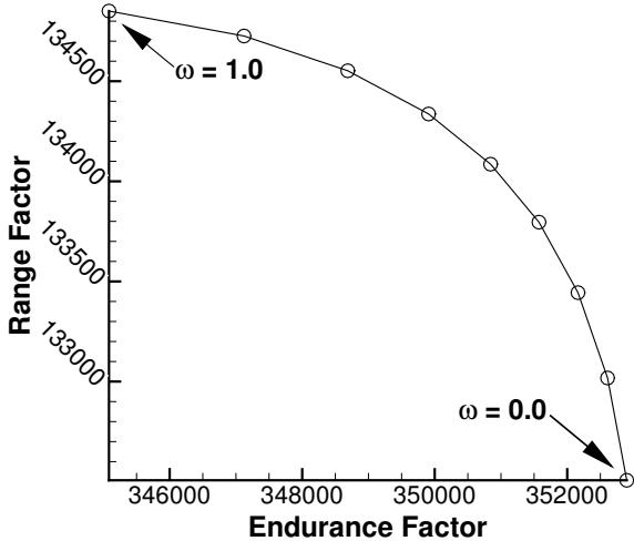
Figure 9. Trade-off between UAV range and endurance performance
