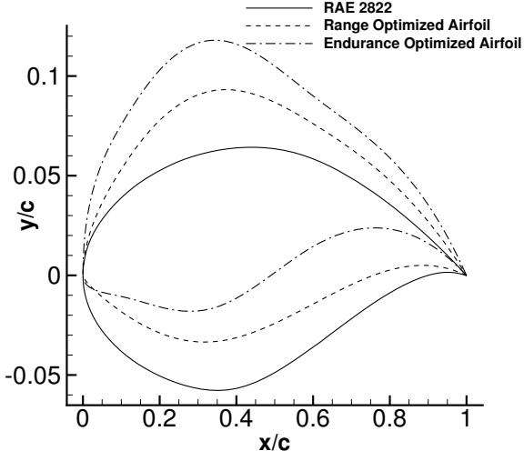
**Figure 4.** A comparison of UAV airfoil geometries for optimal range and endurance performance
