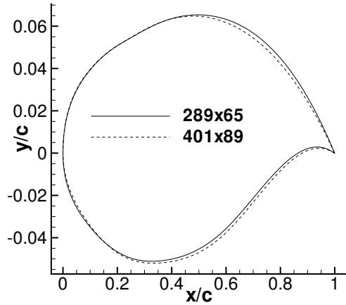
Figure 13. Comparison of optimal airfoil geometries obtained using different grid densities
