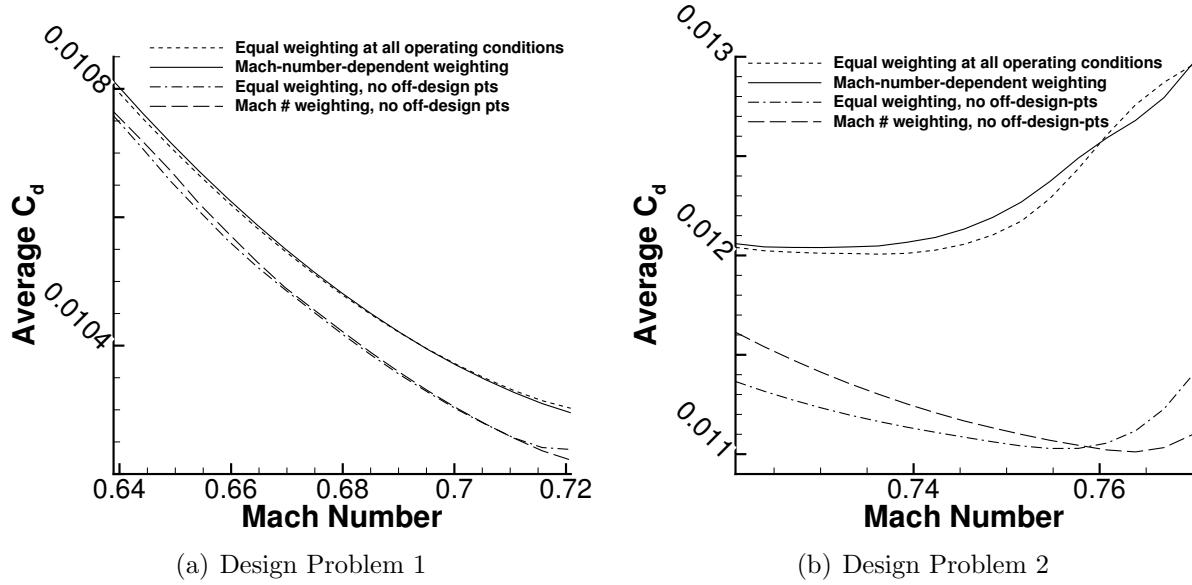
Figure 2. Comparison of average  $C_d$  over the range of aircraft weights versus Mach number obtained using different designer-priority weighting functions
