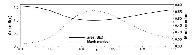
Figure 4: Duct area and Mach number for the quasi-one-dimensional-Euler flow example.
