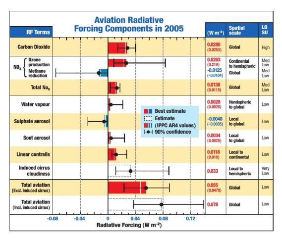
Figure 4: Radiative Forcing (RF) from aircraft, source: [60]
