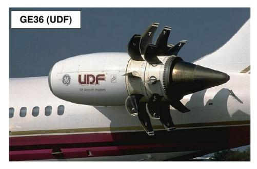
Figure 11: The open rotor concept (experimental GE36 engine), source: [3]
