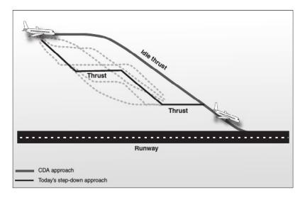
Figure 7: Continuous vs step-down approach profiles, source: [28]
