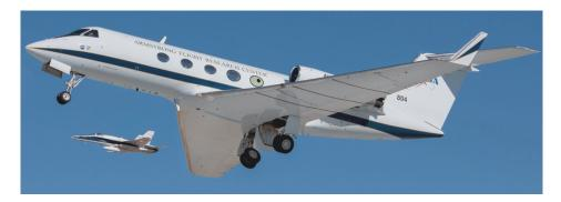
Figure 10: The FlexSys morphing wing geometry on a Gulfstream III flight test aircraft with no external flap-track or distinct control surfaces under the wing, source: [40]
