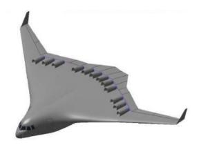
Figure 13: Distributed propulsion system on the CESTOL blended wing-body, source: [48]
