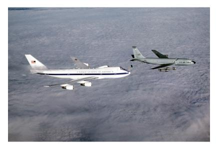
Figure 9: Air-to-air refueling operation, source: [97]
