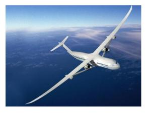
(d) Strut-braced wing design, source: [21]
